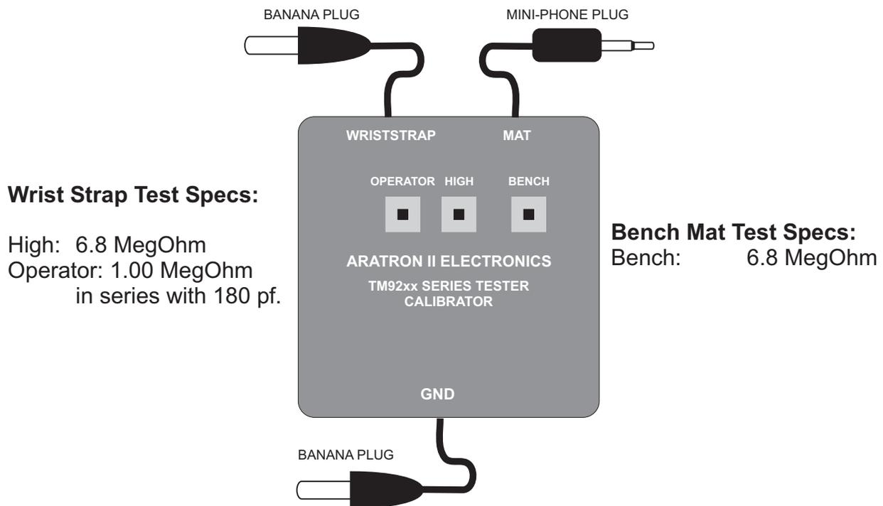
1. Connect the TM92xx Tester ground wire to the ESD Common Point Ground.
